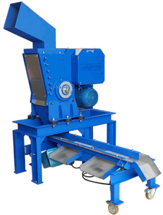
LMFC250 fine crusher with sieve street for dividing the output of the machine by size
