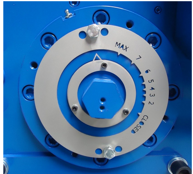
Fine Crusher gap adjustment
