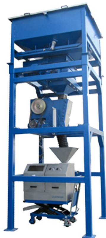
Sampling installation with a LMFC250 fine crusher
