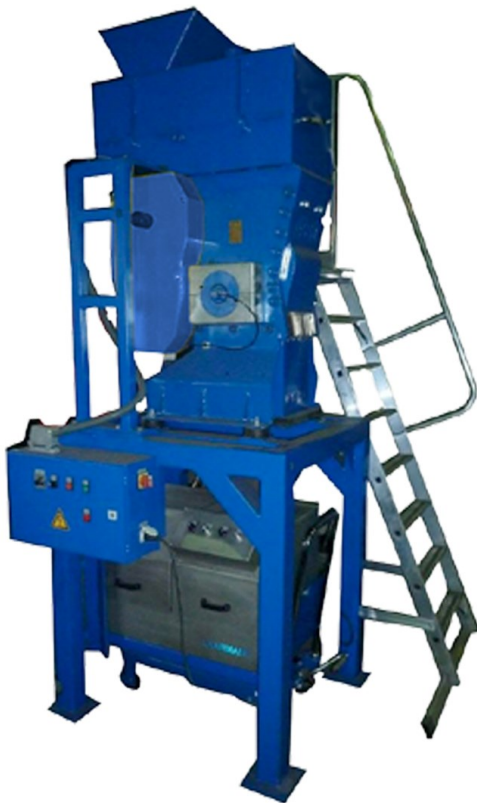
Sampling installation with a LMFC250 fine crusher
