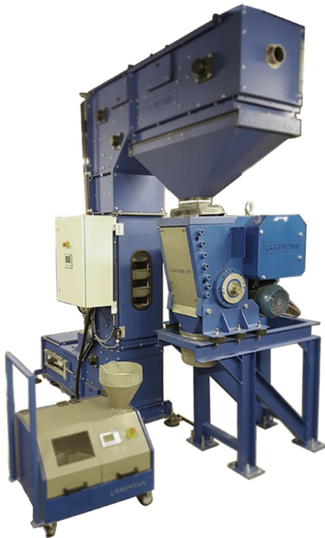
Ferroalloy crushing installation for sample preparation
